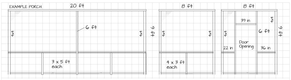
Sketch an elevation of each side of your porch. Note the horizontals and verticals. How many verticals are above the rail? How many are below? Note posts and rail sizes — 4x4 or 2x4. Depending on your screening system of choice, the exact materials and components will vary.
