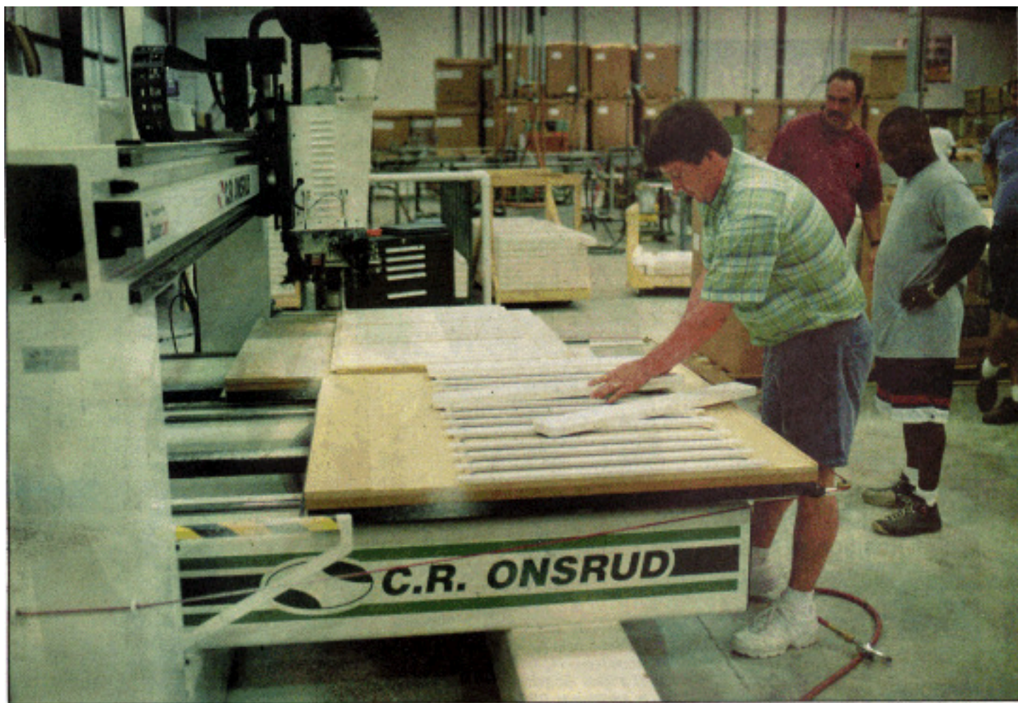
Screen-Tight has invested in sophisticated computerized furniture milling equipment to boost efficiency in the production of door-frame components.
