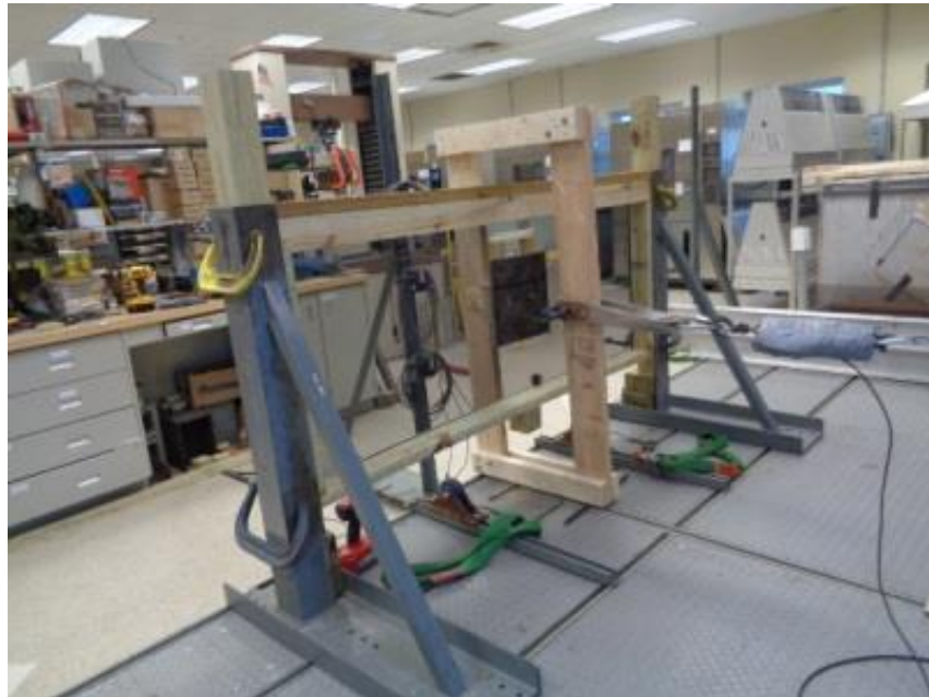
Photo No. 1 In-Fill Load Test at Center of Screen Mesh
