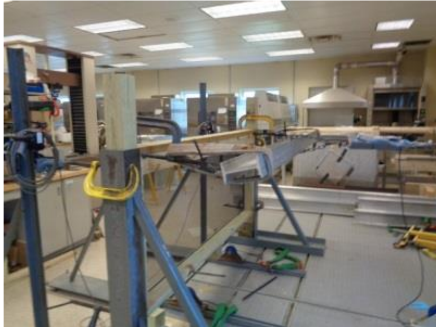
Photo No. 3 Concentrated Load Test at Ends of Top Rail (Brackets)
