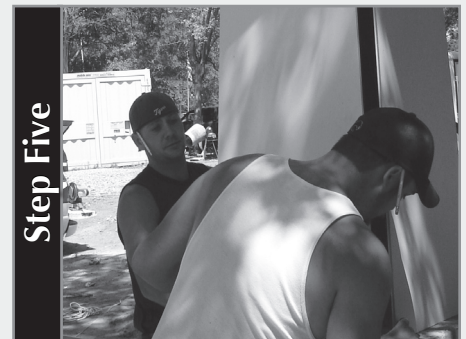
Step Five Then snap 2 halves together after applying small bead [1/16"] of adhesive, forming Tapered Column. [Note: An excessive amount of adhesive in the snap lock may result in a sink line in the outside surface.]
