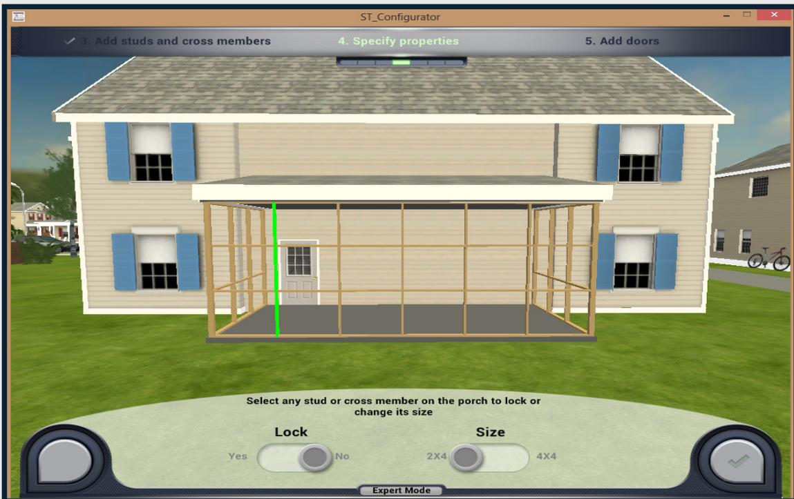
11. You can change the size of individual studs or cross members as needed. Lock a stud or cross member in place.
